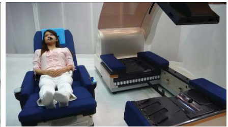
A Robotic Bed poster at the HCR exhibition. It says: The bed turns into a wheelchair while the user stays in bed; It not only helps people with limited mobility to lead an independent life but also reduces burden of care workers.
