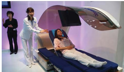
A Robotic Bed poster at the HCR exhibition. It says: The bed turns into a wheelchair while the user stays in bed; It not only helps people with limited mobility to lead an independent life but also reduces burden of care workers.
